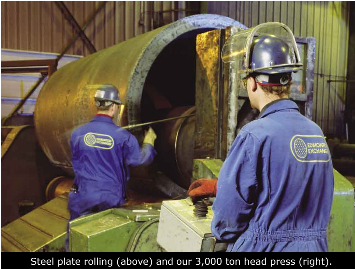
Steel plate rolling (above) and our 3,000 ton head press (right).
