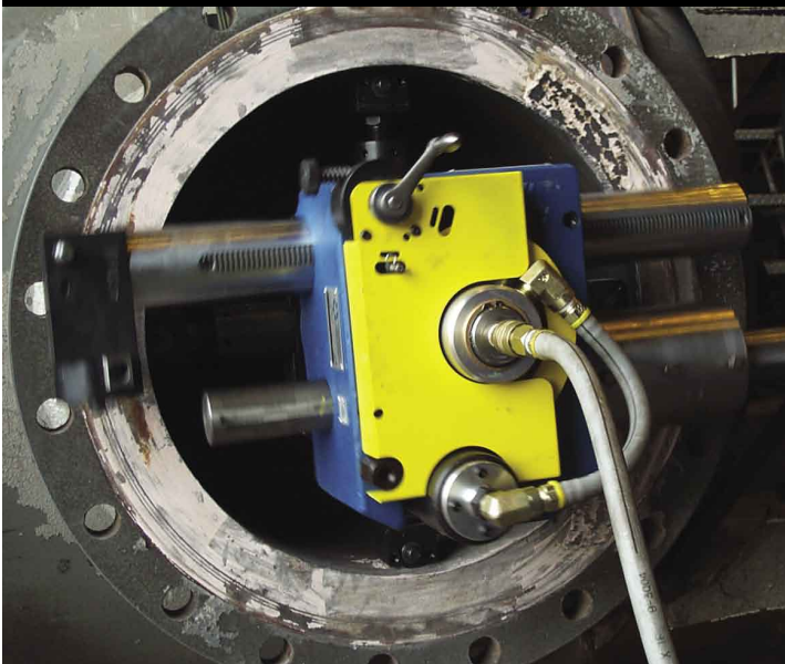
Flange facing in progress (below left) and the fully machined flange face (below right).
