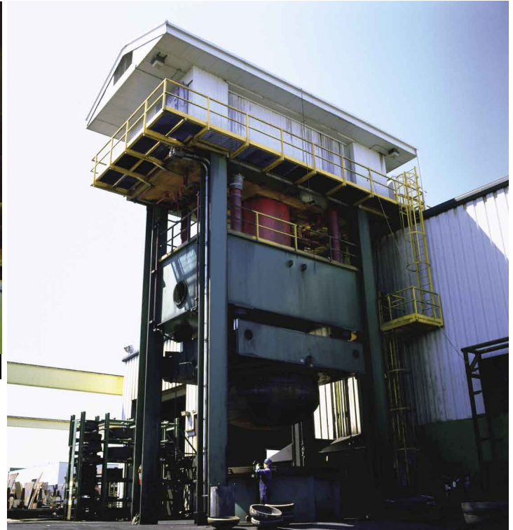
Steel plate rolling (above) and our 3,000 ton head press (right).
