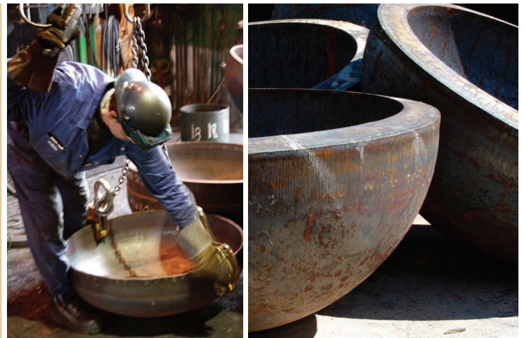
An operator hot spinning a large head (above).
