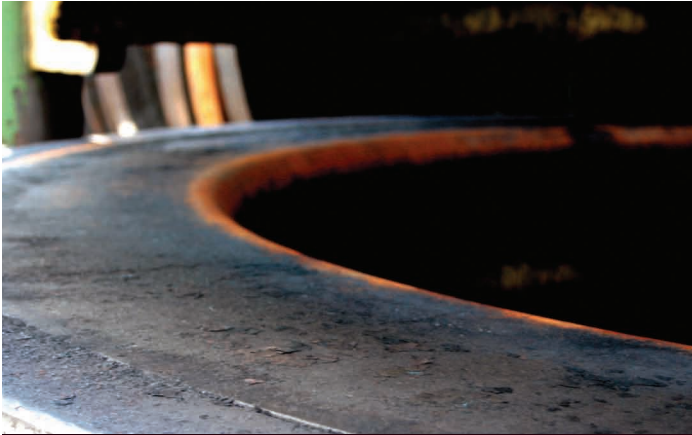
A section of a die on the 3,000 ton head press (above), spinning of a large stainless steel head (below).
