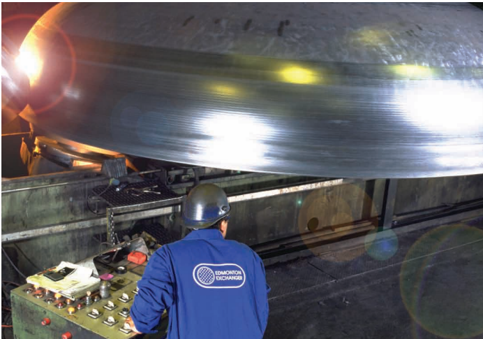
A section of a die on the 3,000 ton head press (above), spinning of a large stainless steel head (below).
