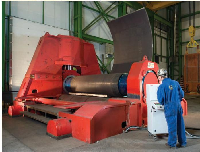
Shells can be supplied with square cut or beveled circumferential and long seams. Long seams can be provided tack welded or fully welded. We can also provide welded circumferential seams by welding together multiple courses.
